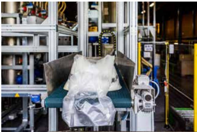
Precise measurements of each ingredient in polymer-based bags are mixed and blended together
