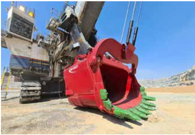
Weir's ESCO® NEXSYS™ GET Lip System for rope shovel dippers
