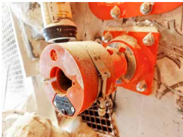
Martin's N2 Position Indicator provides data on the condition and performance of each belt cleaner.
