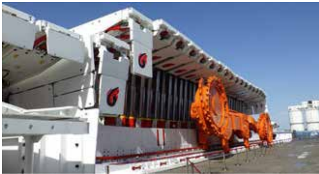
Figure 11: Complete set of fully mechanized mining equipment for super-large mining heights.
