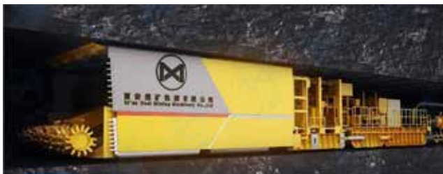
Figure 12: Shield-type intelligent tunnelling robot system.
