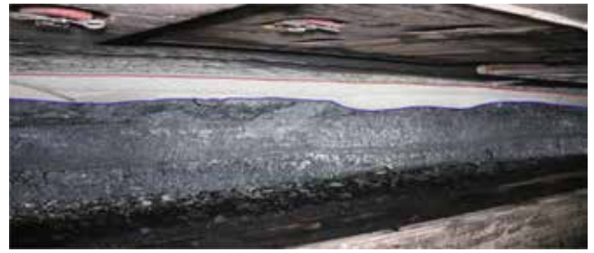
Figure 8: Coal and rock boundary of 1.1-m thin coal seam working face.
