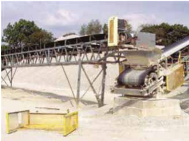
No guard can improve safety if it's not re-installed after service [Image courtesy of the United States Mine Rescue Association]
