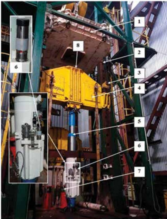
**Figure 7:** Drop-weight tester for valve's opening time; 1-impact weight (20,000 kg), 2-impact guiding gear, 3-traverse blocking pin in the station frame, 4-traverse (3300 kg), 5-double-telescopic hydraulic leg, 6-tested safety valve, 7-pressure sensor, 8-height of drop.
