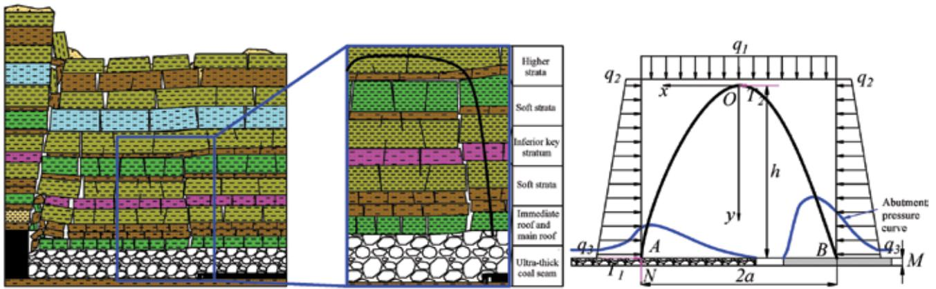
Figure 15: Relationship between support and surrounding rock under roof arch bearing structure.
