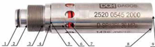
**Figure 5:** Construction of a piston safety valve with a gasket and spring pressure: 1-round seal, 2-connection stub, 3-round piston seal, 4- piston, 5- piston pressure plate, 6-casing, 7-spring, 8-thrust plate, 9-adjustment screw.
