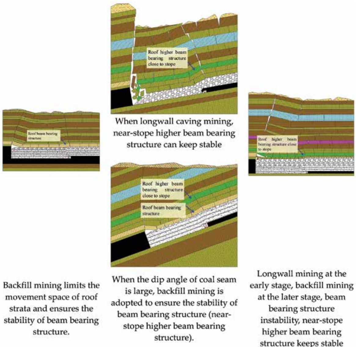
typical ultra-thick coal seam in Xinjiang is studied. In the process of multi-layer mining, the roof bearing structure shows the evolution process of “beam structure-higher beam structure-arch structure”. At the early stage of multi-layer mining, the load on support is rotary subsidence load of the near-stope roof bearing structure and gravity
