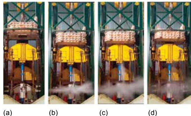
**Figure 8:** Phases of the tested leg loaded with mass impact (140.0 kJ); initial impact weight drop (a); the safety valve opens (b); liquid outflow from the leg (c); the safety valve closes (d).
