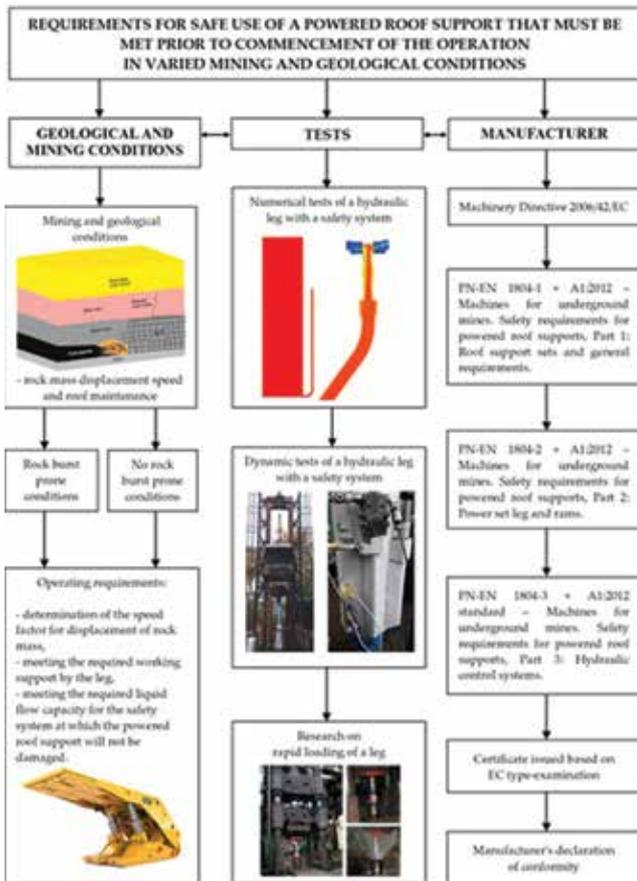
Figure 15: The concept of the procedure for admitting the powered support to be installed and operate in longwalls characterised by varied mining and geological conditions.
