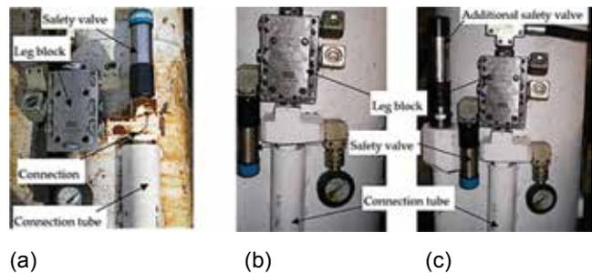
**Figure 6:** Exemplary solutions of systems protecting hydraulic legs with liquid outlet outside the hydraulic system of the support; with one valve, a universal safety system (a); a system for deformation impact of the rock mass (b); a system protecting against dynamic overload (c).
