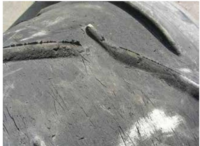
Chevrons as high as 25mm or 32mm can wear almost completely flat in a remarkably short time.
