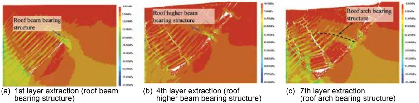
Figure 17: Evolution process of roof bearing structure of inclined ultra-thick coal seam (coal seam dip angle 45°).
