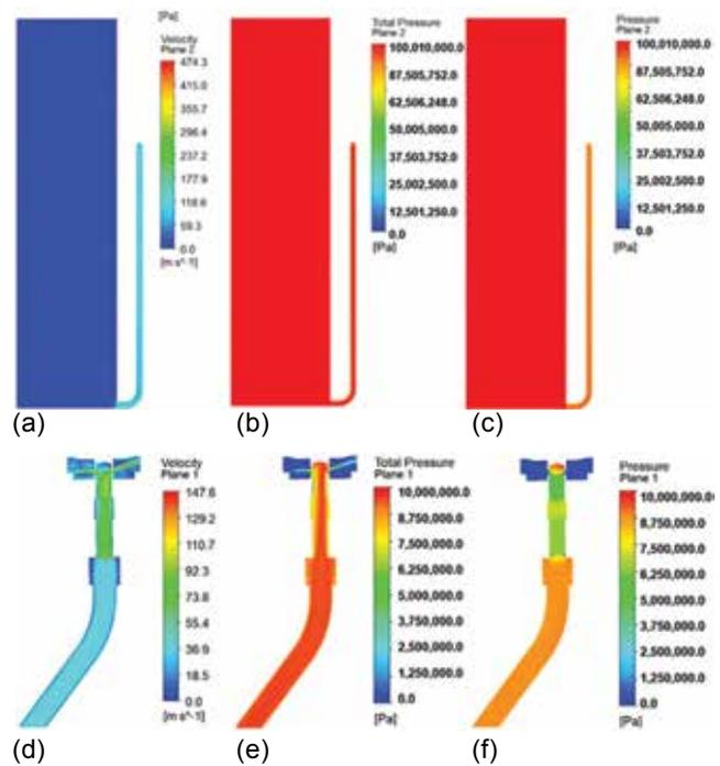
**Figure 12:** Distribution of velocity (a), static pressure (b) and total pressure (c) in a hydraulic leg and flow velocity (d), total pressure (e) and static pressure (f) in the connection supplying liquid to the safety valve at static load on the leg.
