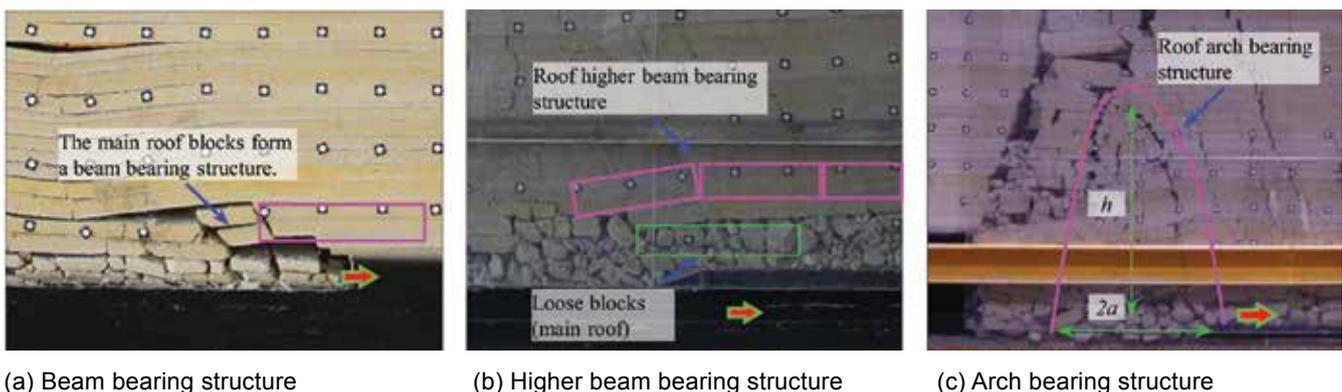
(a) Beam bearing structure
