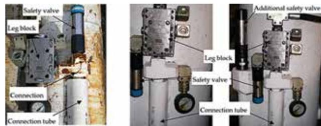
**Figure 6:** Exemplary solutions of systems protecting hydraulic legs with liquid outlet outside the hydraulic system of the support; with one valve, a universal safety system (a); a system for deformation impact of the rock mass (b); a system protecting against dynamic overload (c).
