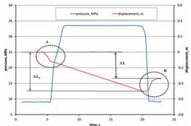
**Figure 11:** Time courses of the value of the displacement (slide-down) and pressure in the tested leg with spring deformation zones marked (A and B) and full slide-down ( $\Delta L_T$ ) (own study based on<sup>20,21,49</sup>).
