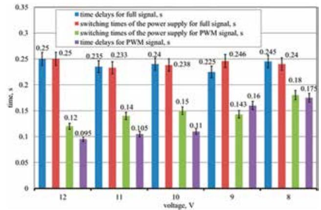
**Figure 14:** Switching on and lag times with the PWM and full signal for leg's sliding down mode (own study based on data from<sup>54,55</sup>).
