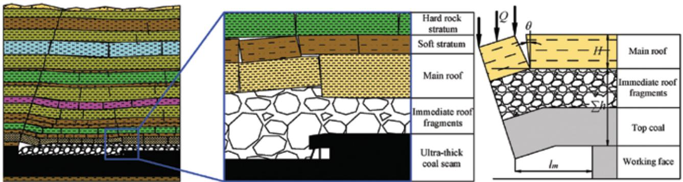
Figure 13: Relationship between support and surrounding rock under roof beam bearing structure.
