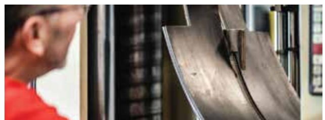
Dunlop's 'Jack the Ripper' rip test in action
