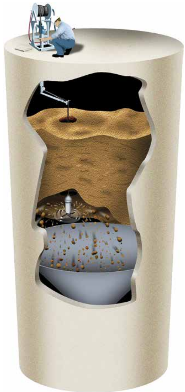
Safe, effective cleaning requires tools that work inside the silo from the top, controlled by personnel outside.
