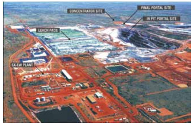
Figure 6: Heap leach facility layout.
