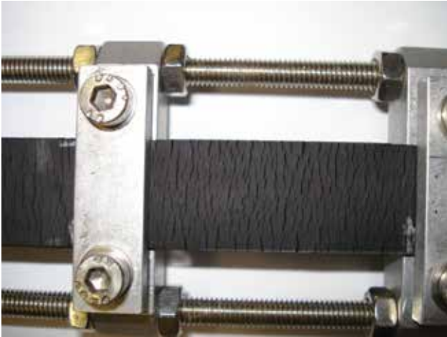
Ground level ozone seriously damages rubber
