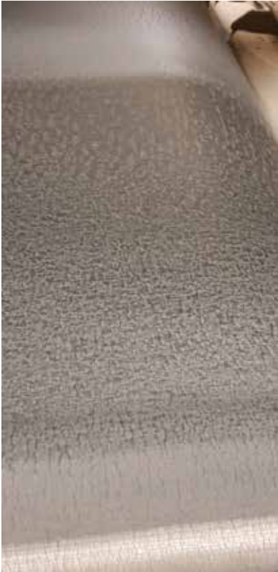
Ozone cracks in the surface of the rubber.
