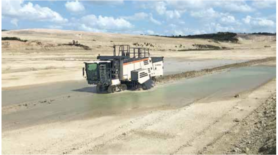
The 220 SMi 3.8 can easily handle difficult conditions – thanks to its adjustable longitudinal and cross slope, larger puddles are no problem for the machine.
