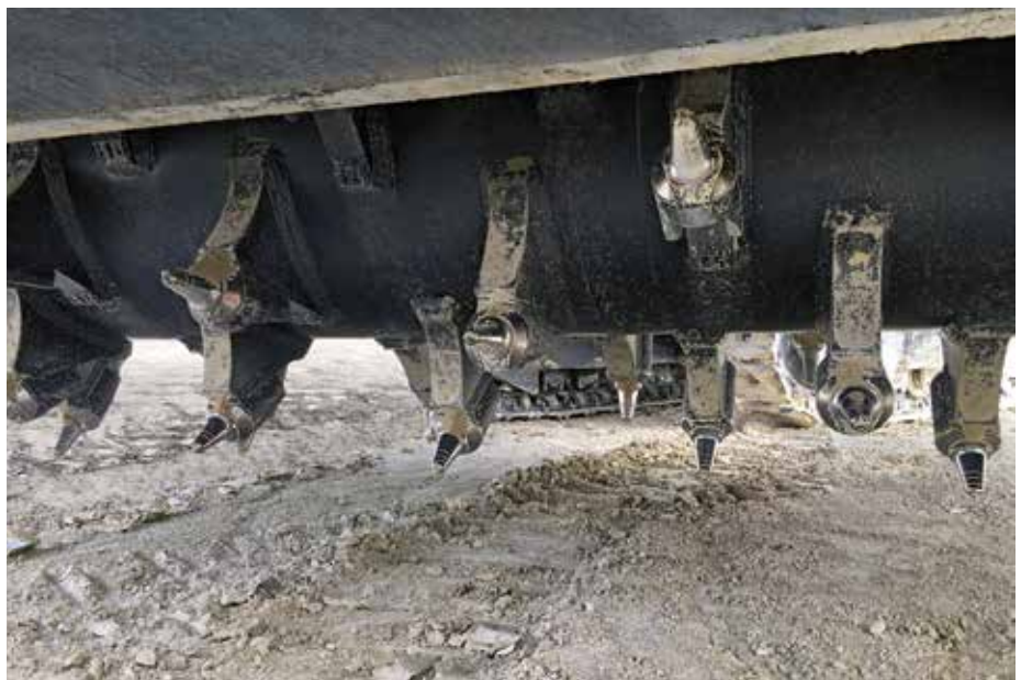
Wirtgen's powerful milling drums can produce significantly smaller grain sizes than, for example, drilling and blasting or, as shown here, using a dozer.
