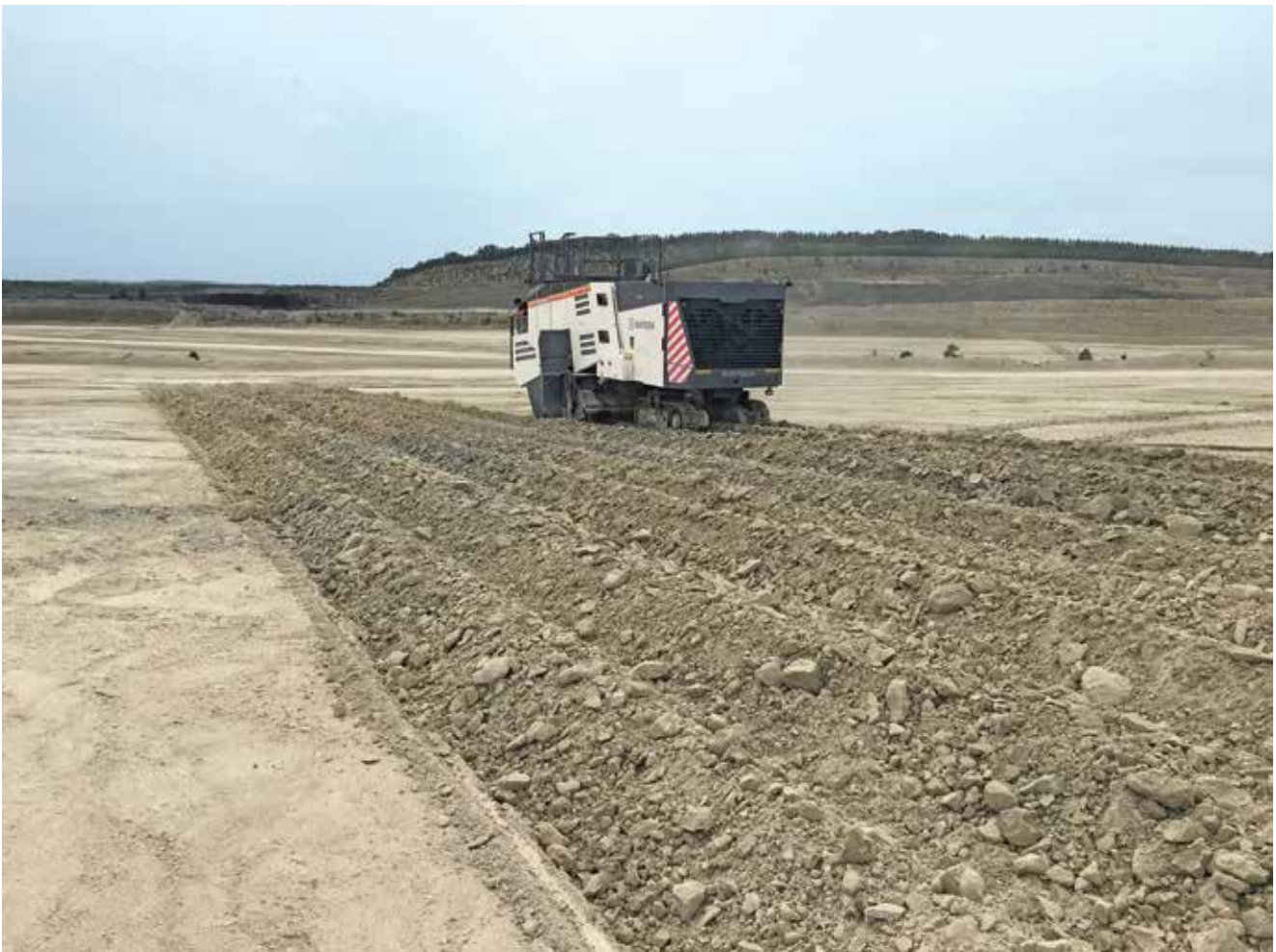
The surface miner mills the material and deposits it behind the machine in a windrow.
