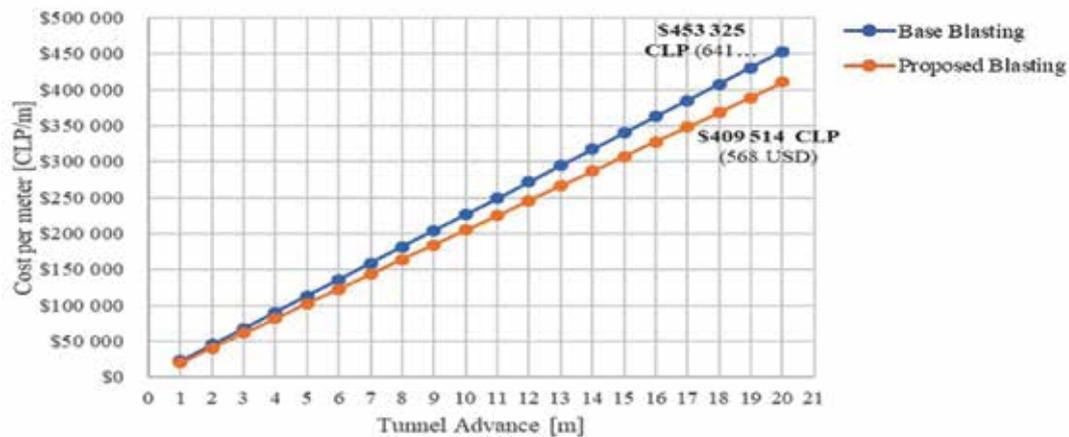
Figure 11: Cost per meter excavated, over 20 blasts.
