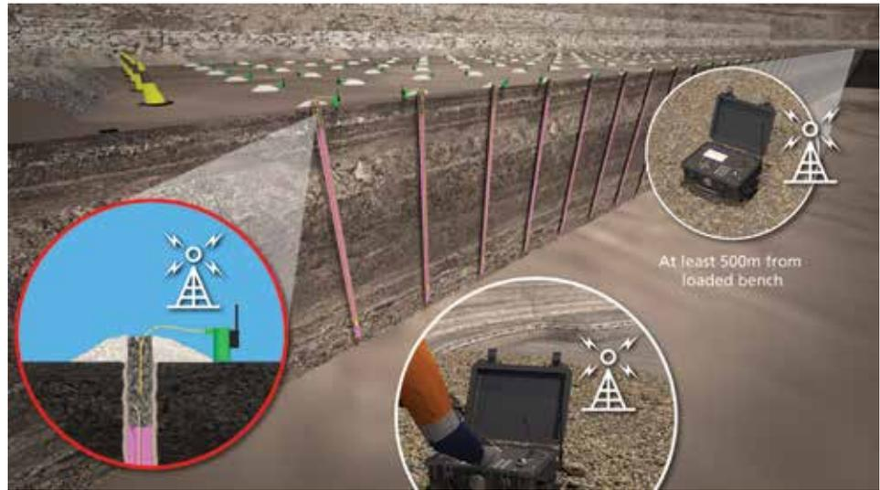
Wireless to the blasthole collar concept is still susceptible to wire damage.
