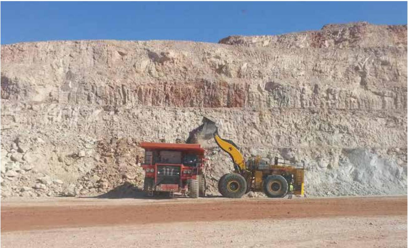
Figure 4: The DE loader filling an AC truck at a rock bench (Özdoğan 2013).
