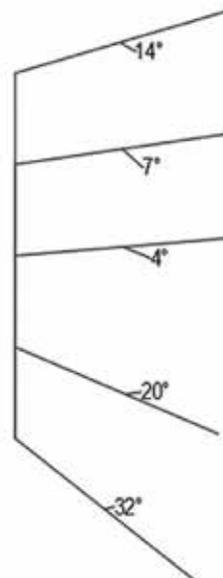
Figure 2: Restructured La Palmera Mine' firing diagram in front and side view.
