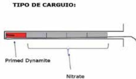
Figure 6: Blast 1: drilling and charging configuration.
