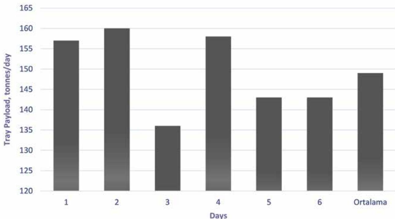
**Figure 5:** Daily tray payload of 150 tonnes trucks loaded by a 21 m<sup>3</sup> loader.
