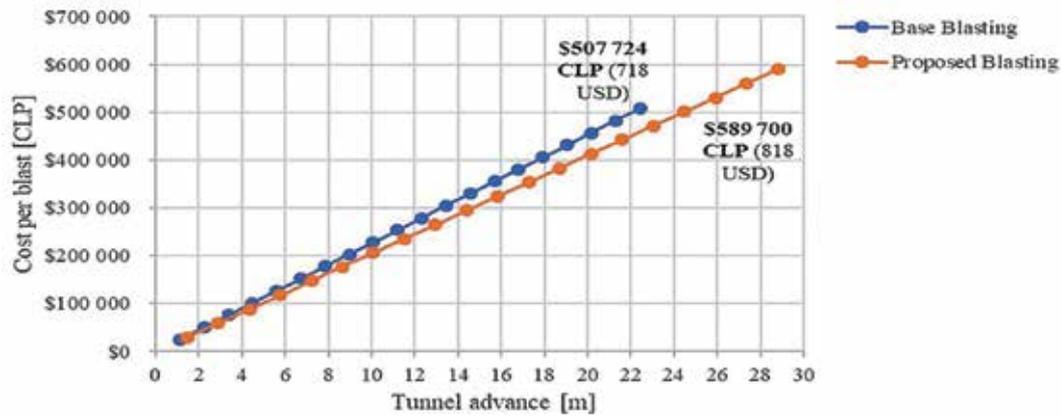
Figure 10: Cost per blast over 20 blasts.
