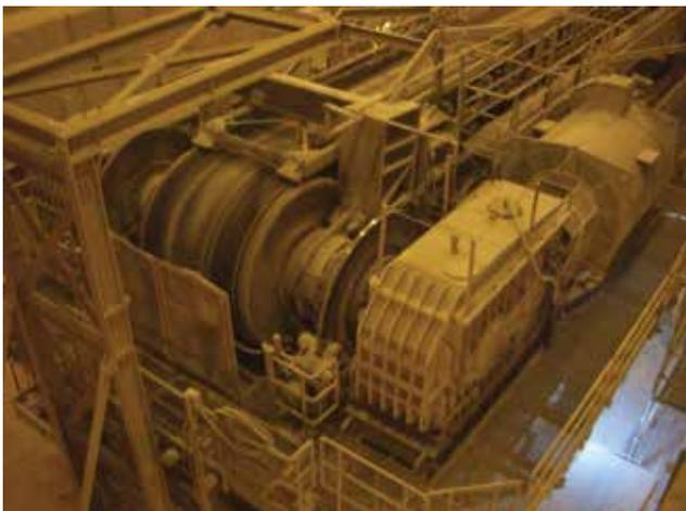
KUMERA conveyor belt drive solution – right position.
