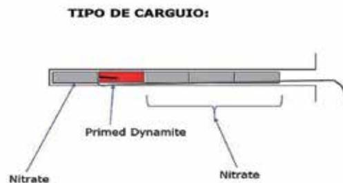
Figure 8: Blast 3: drilling and charging configuration.
