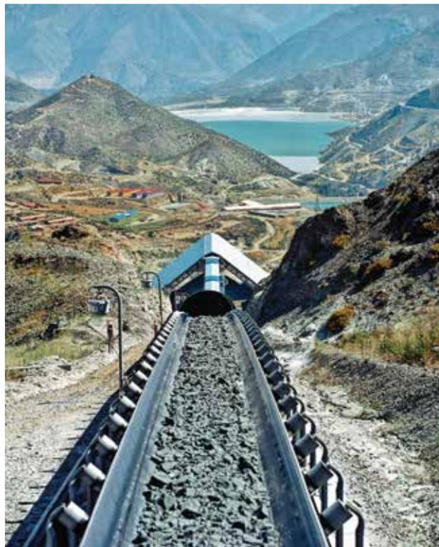
Conveyor belt slope downwards – generator mode.
