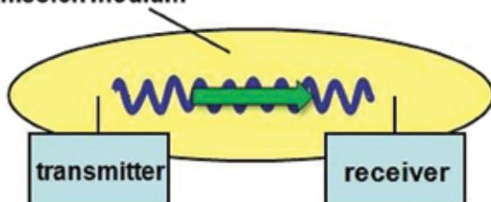
Components of a simple wireless communications link.
