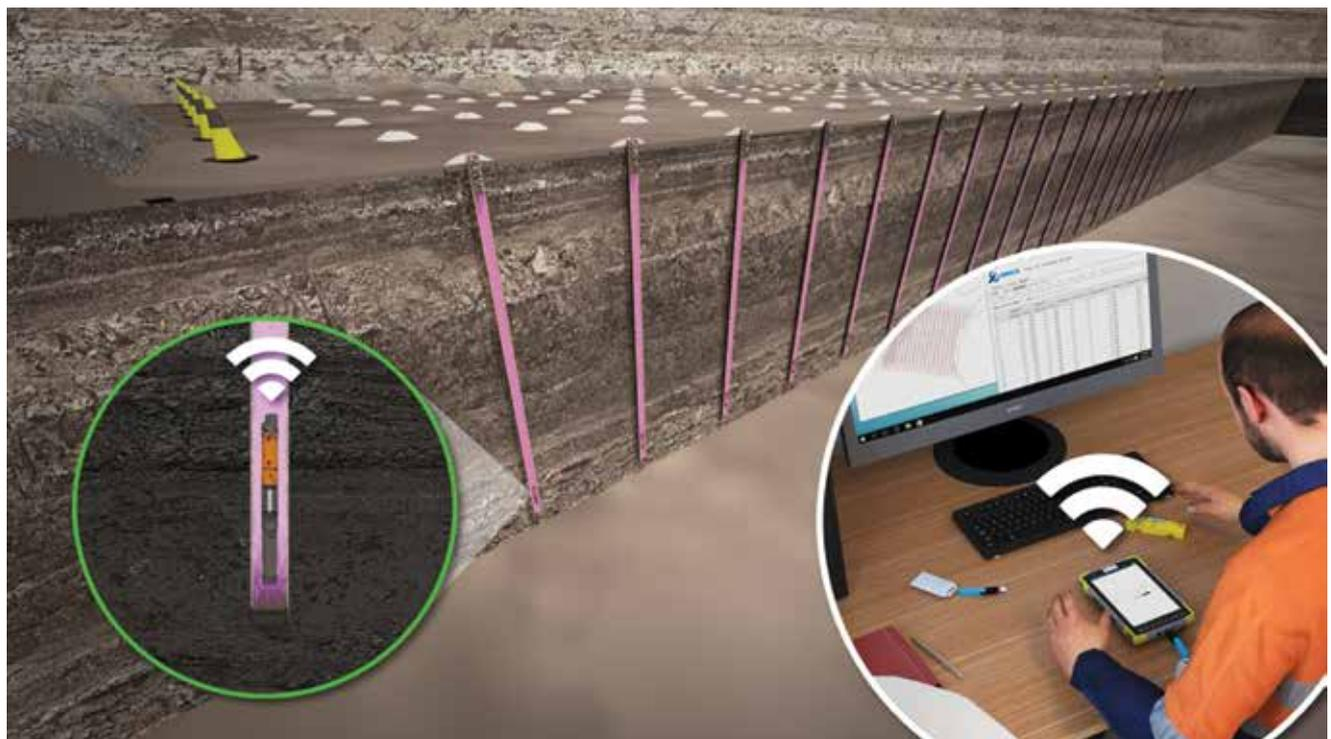
WebGen™, the world's first fully wireless initiating system has no downlines and surface connections to the detonator.
