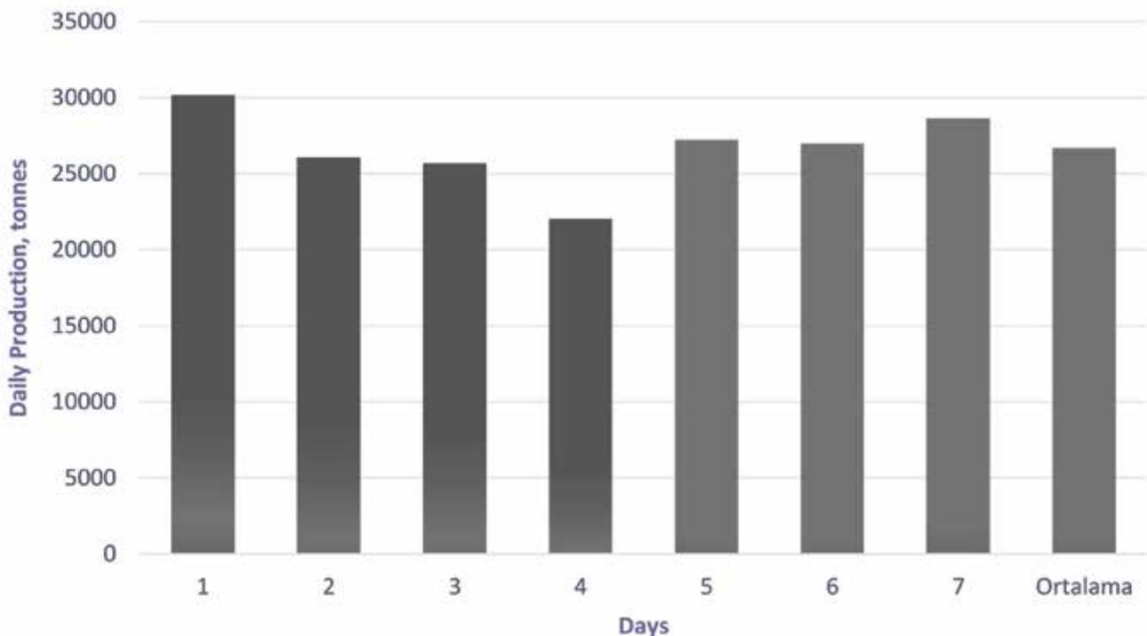
**Figure 6:** The 220 tonnes trucks' average daily production in a week's time.
