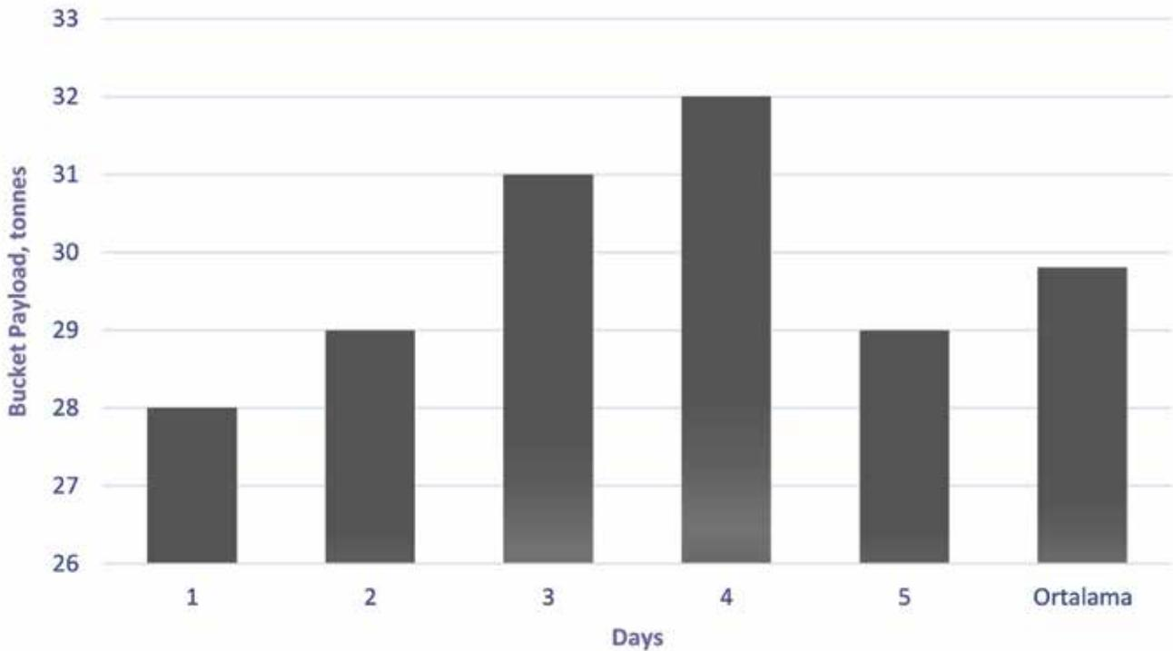
Figure 3: Payload variation of a 21 m<sup>3</sup> a DE loader in a five days of operation.
