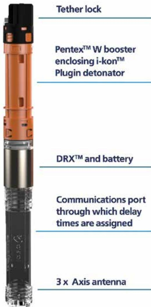
WebGen™ uses ultra low-frequency magnetic induction signals to transmit firing commands.
