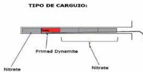
Figure 7: Blast 2: drilling and charging configuration.
