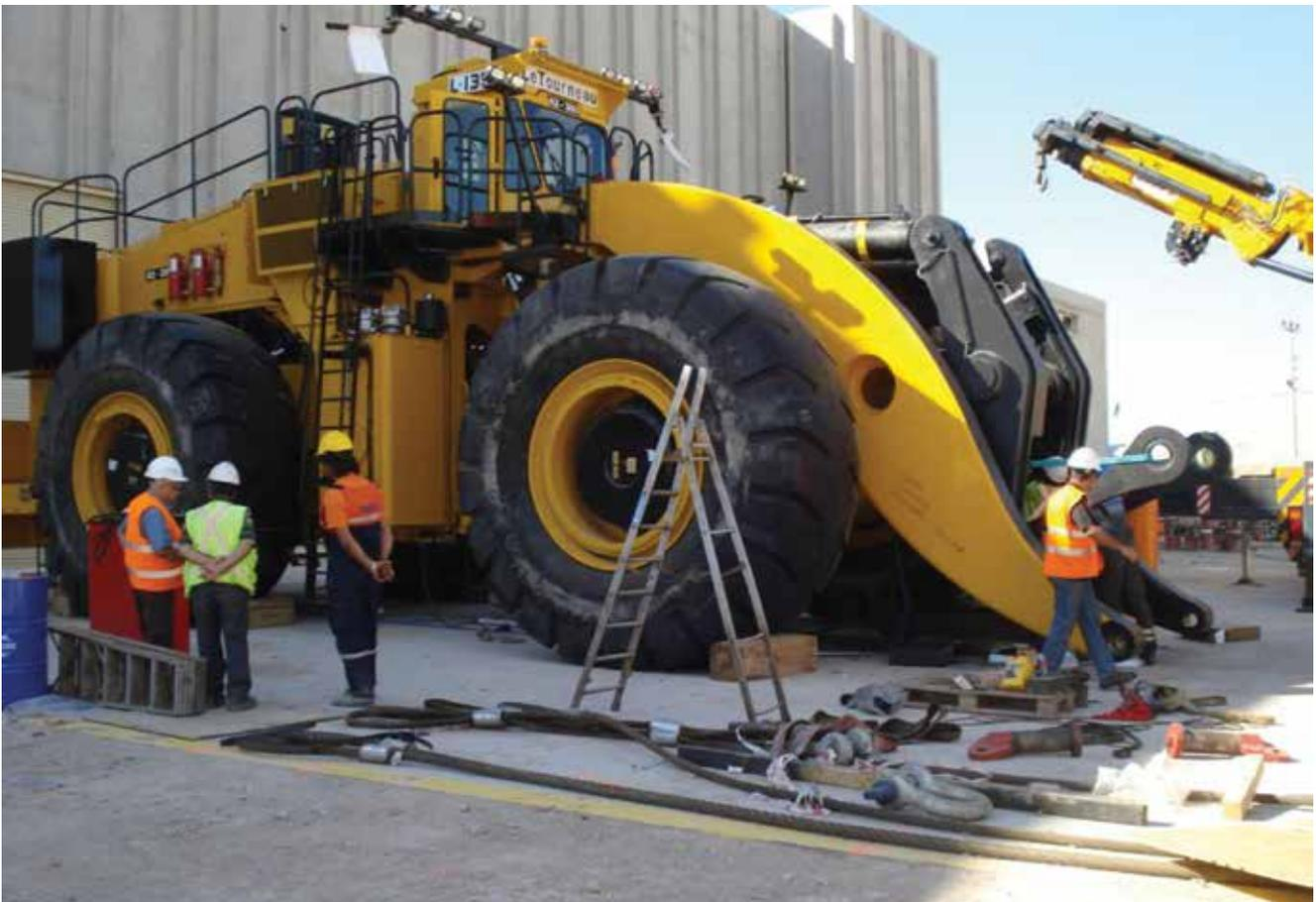
**Figure 1:** Erection of a 21 m<sup>3</sup> mining loader in workshop yard (Özdoğan 2013).
