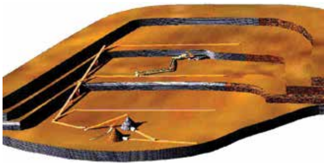
Figure 2: Multi bench operation.
