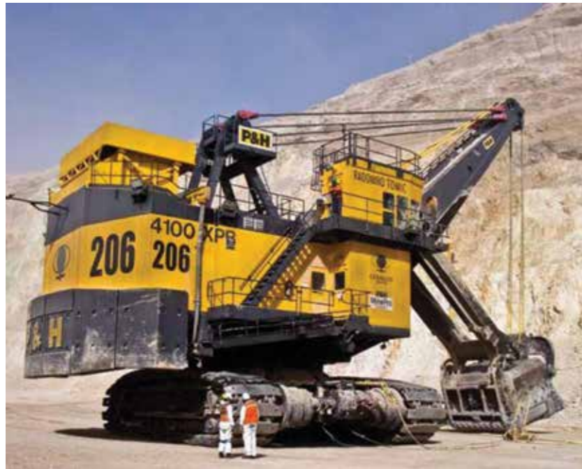
Electric rope shovels with capacities up to 100 tons are one of the most critical assets in open pit mines.
