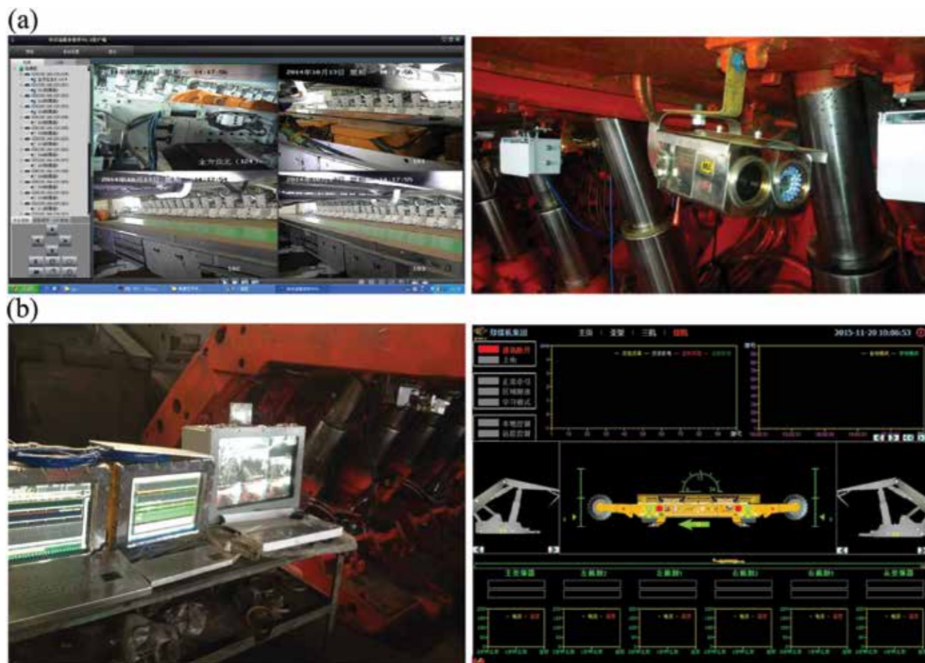
Figure 2: The key equipment in automatic cutting: (a) video surveillance system; (b) shearer remote control system.
