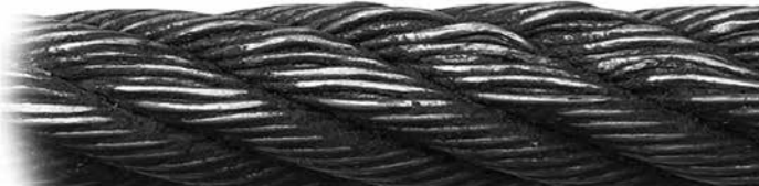
“CRUSHING” > Typical example of external pressure on a wire rope.
