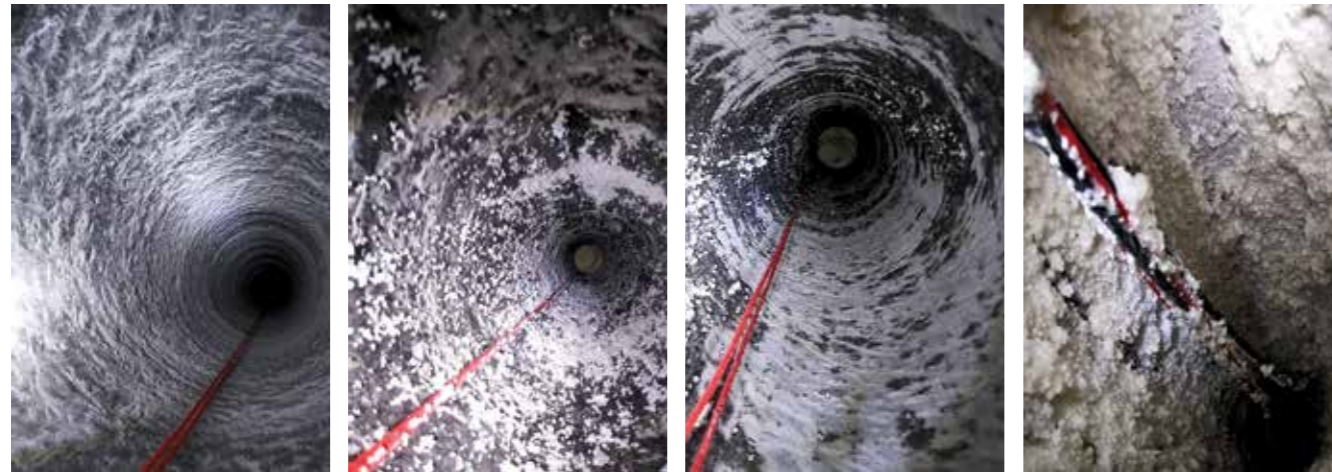
Figure 2: Increased clinging of explosives on a blasthole wall as the percentage of emulsion in the blend increases.
