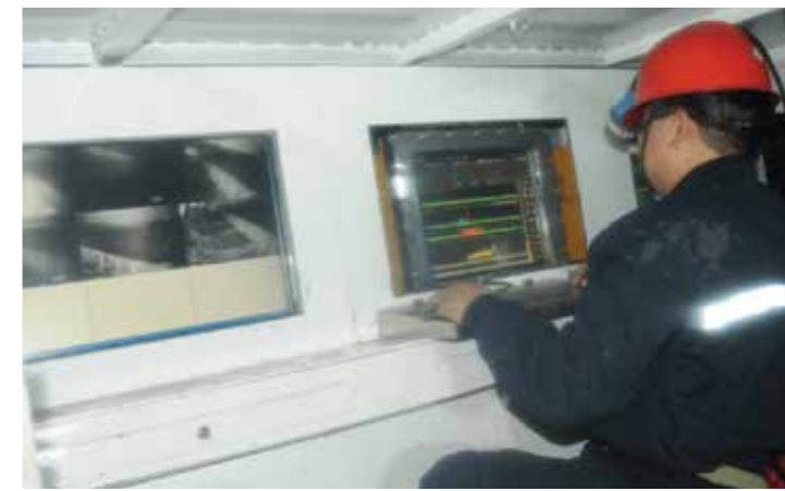
Figure 5: Shearer operation through remote control system.
