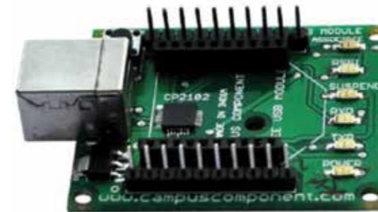
Figure 17: Zigbee USB interfacing Board
