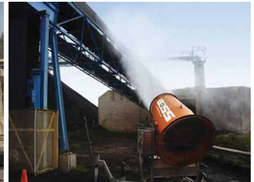
The DustBoss DB-60 is an oscillating, twenty-five horse-power fan that can cover 21,000 square feet with a blanket of fine mist. Photo courtesy of Dust Control Technology.
