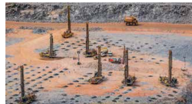
The ARDVARC control systems use AsteRx-U receivers, which run advanced GNSS+ algorithms including IONO+ for robust operation in areas of intense solar activity.
