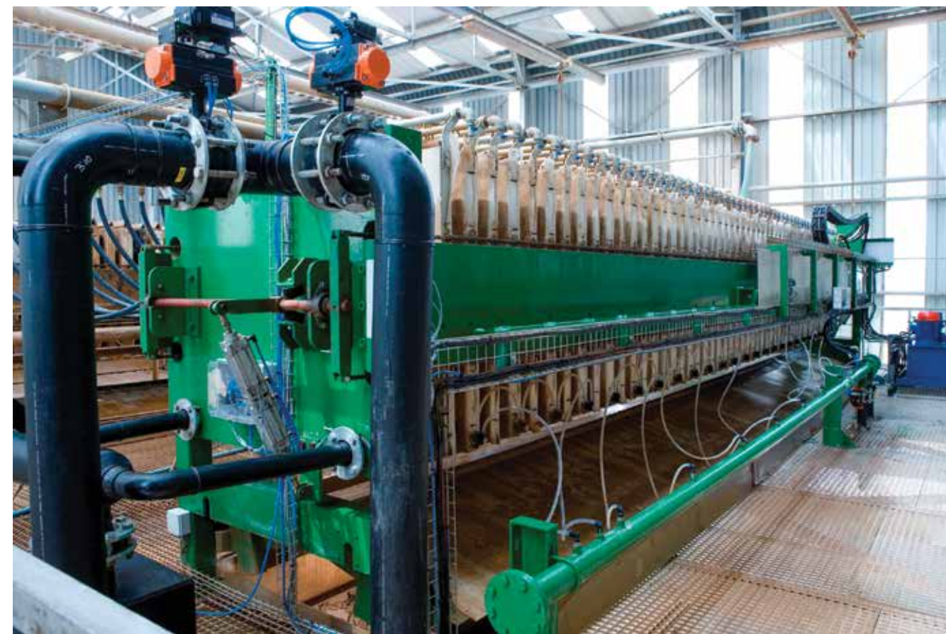
The arsenic sludge from the HDS is dewatered by filter press while the solid cake is disposed of.
