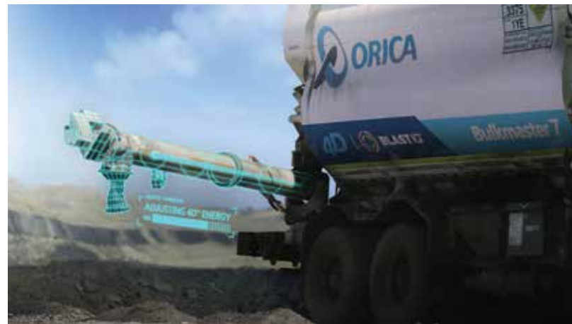
Unique emulsion blended with porous prills enables augered explosives loading in dry and dewatered holes which is much faster than pumped loading.
