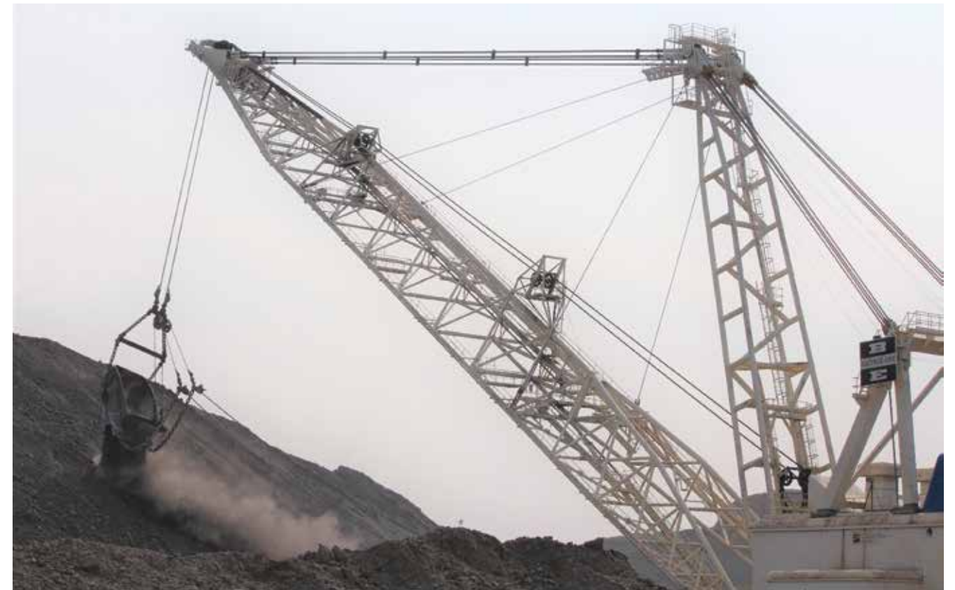
A Bucyrus 1570 Dragline Equipped with Applied Fiber Synthetic Main Boom Support Pendants.
