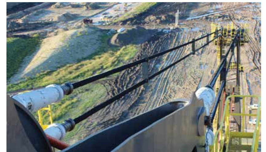
Looking down from the Boom Tip- Applied Fiber Pendants on Marion 8200 Dragline.
