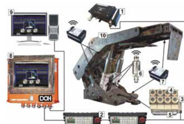
Figure 3: Prototype devices that are part of the system; 1 – intrinsically safe power supply, 2 – controller, 3 – electro-hydraulic executive block with control inserts, 4 – solenoid valve, 5 – control bar, 6 – pressure sensor, 7 – inclinometer, 8 – underground computer, 9 – surface computer, and 10 – powered roof support section.
