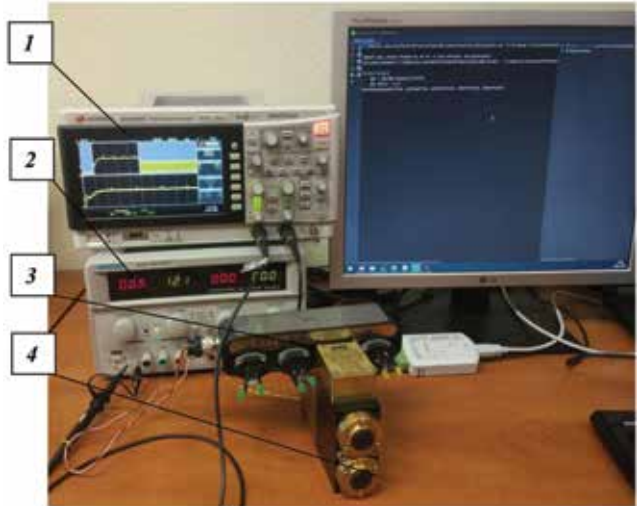
Figure 6: Test monitoring equipment, where 1 – oscilloscope, 2 – laboratory power supply, 3 – controller module, and 4 – solenoid valve.
