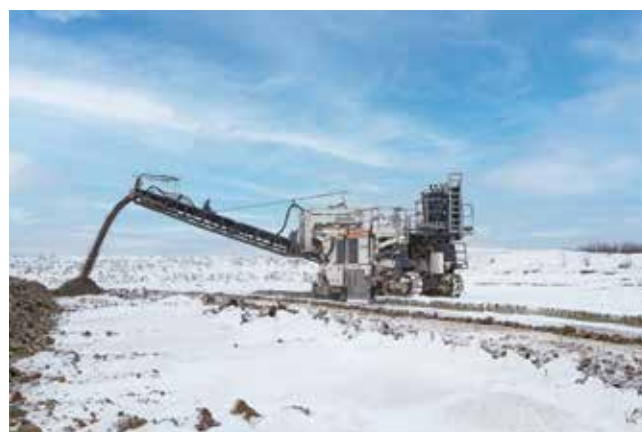
With the 280 SM(i) surface miner, primary resources are extracted in purest quality and crushed in situ in a single operation – without drilling and blasting, and with minimal environmental impact.
