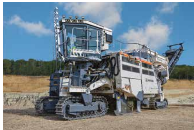
The Wirtgen 280 SM(i) is a high-performance surface miner for reliable, selective extraction of primary resources by direct loading, sidecasting or cut-to-ground.
