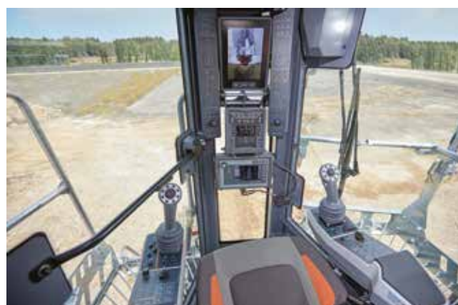
The 280 SM(i) surface miner's air-conditioned and soundproofed operator's cabin with all-round glazing is swivel-mounted on the front chassis column and provides a productive working environment with a low risk of fatigue.
