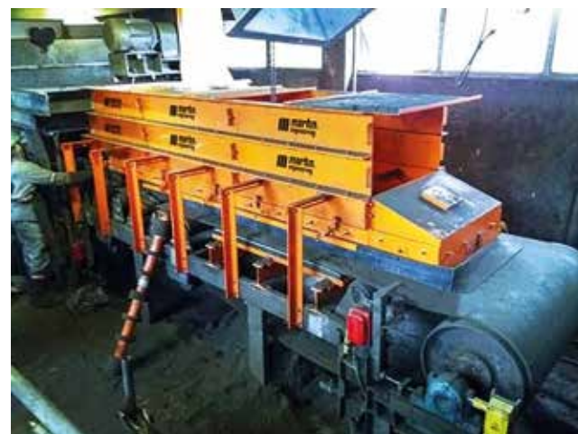
Figure 1: With the proper enclosure design, dust volumes can be lowered to below regulatory levels.
