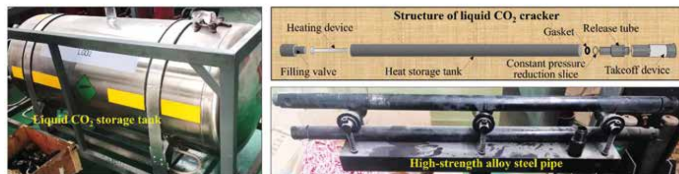
Figure 8: Liquid CO 2 storage tank and cracker.
