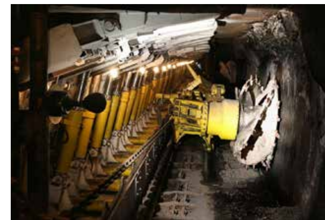
Figure 1: The diagram of the shearer, AFC, and roof support system.
