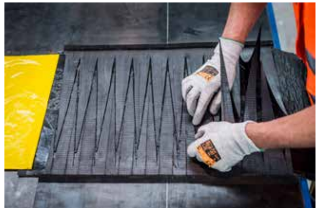
Finger splice joints are much stronger and reliable.
