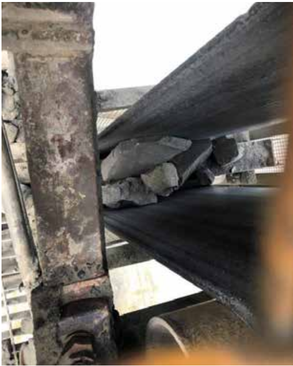
Trapped granite buckled the conveyor, but the UsFlex belt kept on rolling
