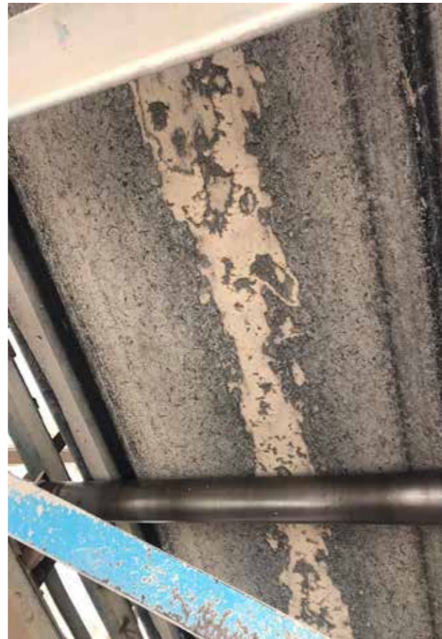
More than 50% of conveyor belts are significantly below the minimum standards claimed by the manufacturer.
