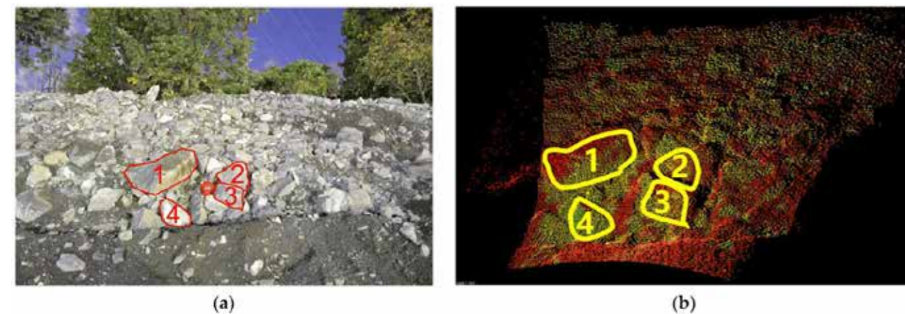
Figure 5: Point cloud processing of mine pile. (a) Mine pile original image; (b) mine pile point cloud image 47 .
