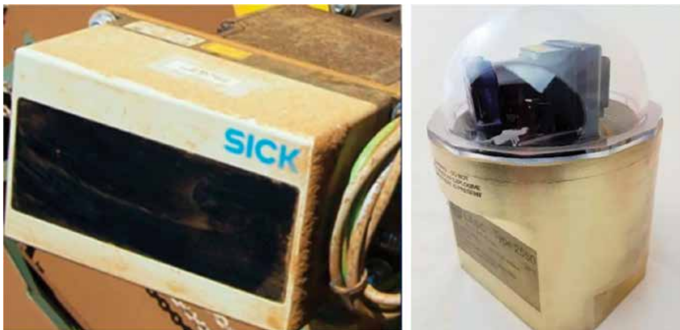
(a) (b) Figure 12: The diagram of (a) the SICK LMS200 scanning laser and (b) ExScan.
