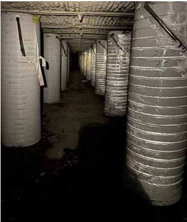
J-CRIB®, a pumpable standing support, provides significant strength and logistical advantages over traditional coal mine standing support.
