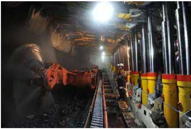
Figure 5: The shearer, AFC, and roof support system across the longwall face in an underground mine.
