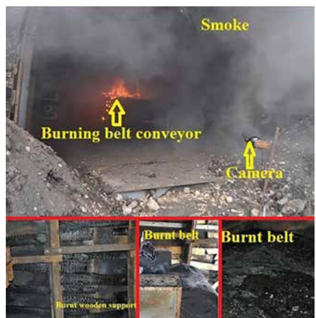
Figure 2: Burning conveyor belt during the experiments, and burnt wood support materials and burnt belt after experiments.
