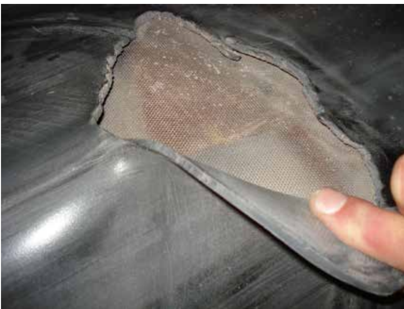
Surface cuts in low grade rubber propagate more quickly and link up with other areas of damage, causing pieces of rubber to detach completely.
