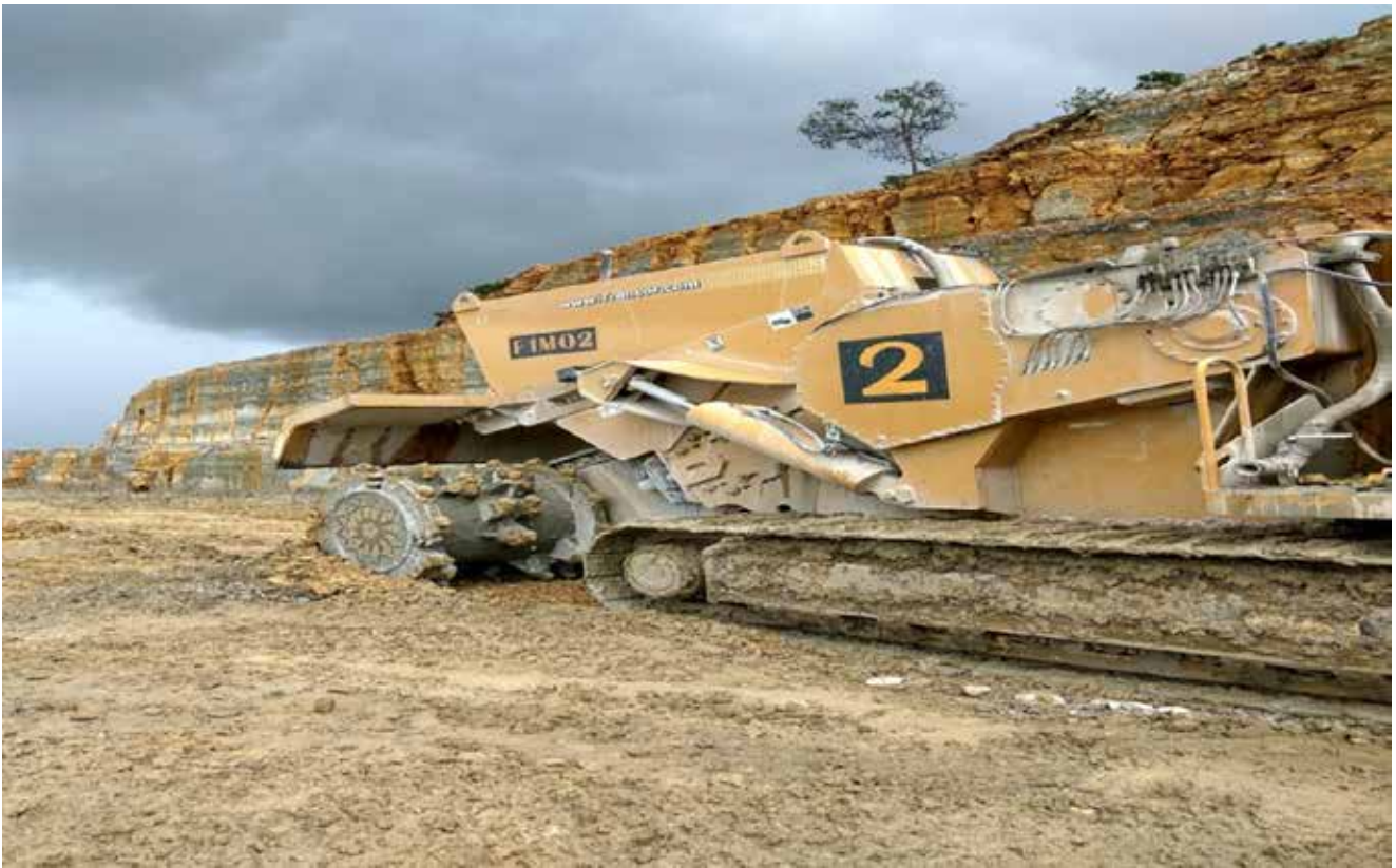
Figure 2: Use of Trenchor Surface Miners (having Top-Down Mechanical mechanism of cutting) in a Limestone Mine of Indonesia having average 80 to 140 MPa UCS.
