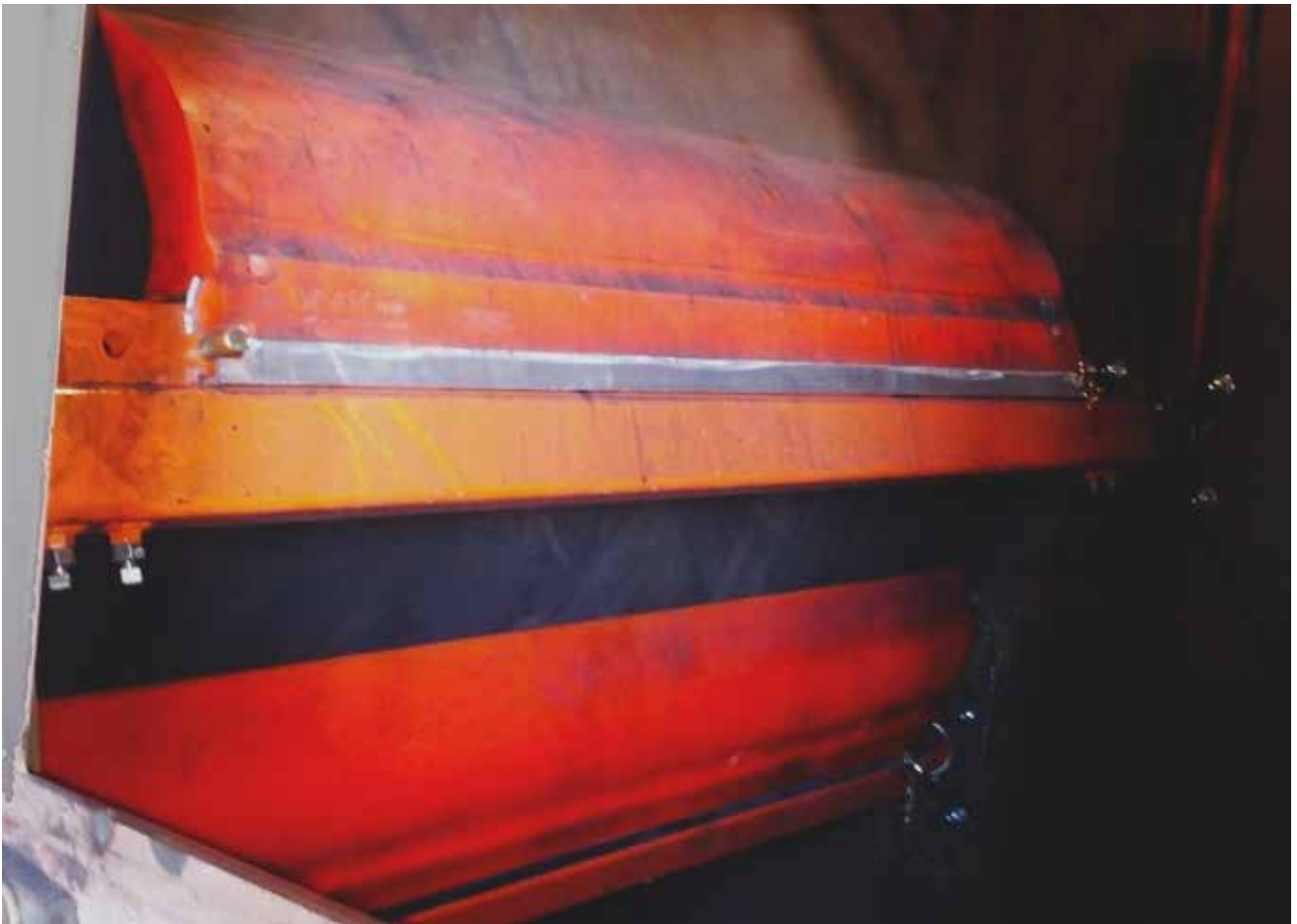
Larger than minimum head pulley diameter for adequate belt cleaning with two primaries and one secondary cleaner.
