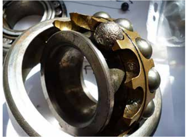
Figure 4: Revealed bearing damage from a teardown inspection.
