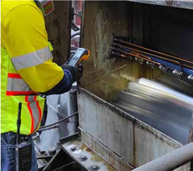
Figure 3: Stroboscope gearbox inspection.
