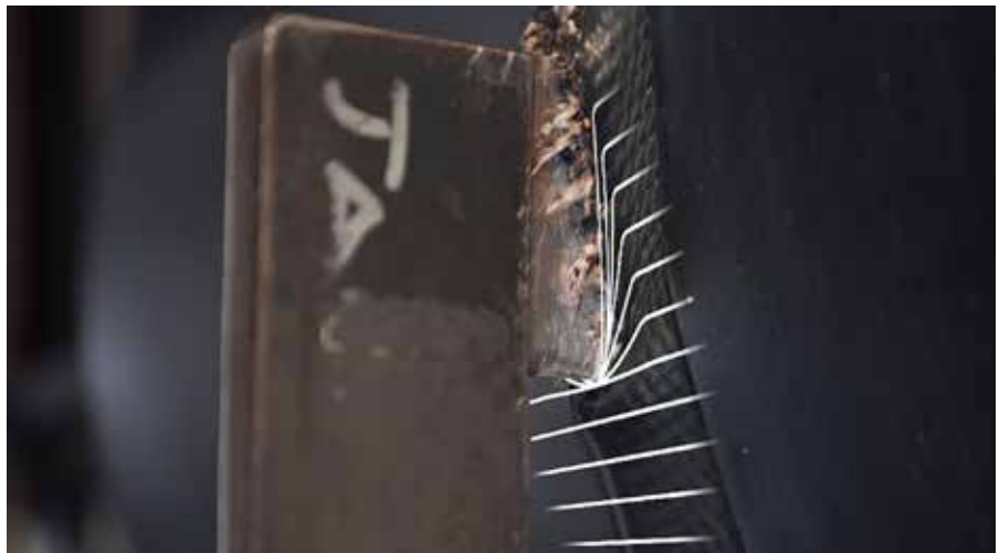
Weft strands bundle together to stop belt or expel penetrating object. (Source: Graphically enhanced image supplied by Fenner Dunlop).
