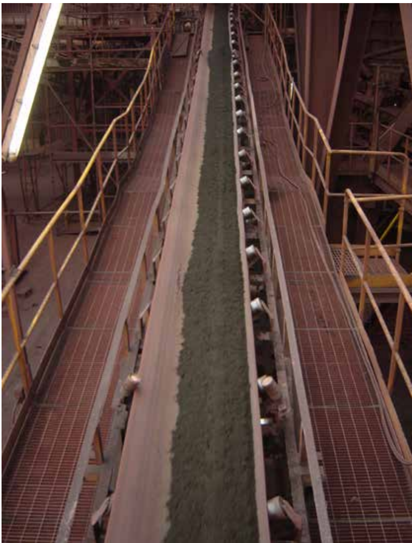
Shifting material causing mistacking
