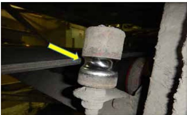
Vertical edge guides act as more of an indicator of mistracking and can create more issues due to severe belt drift.
