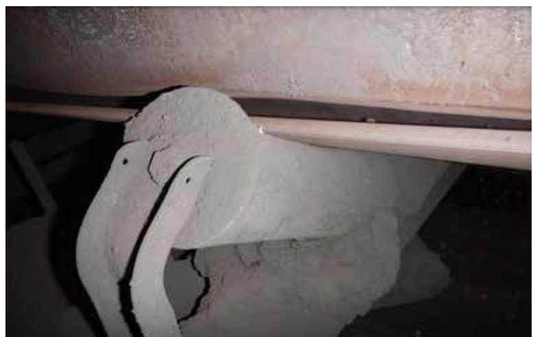
A seized idler wears down from belt friction, creating a potential fire hazard.
