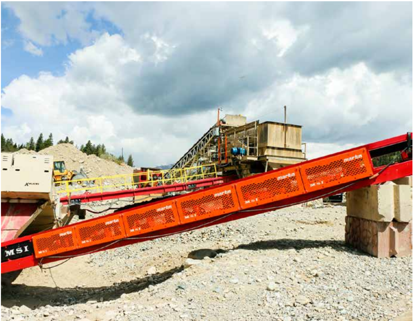
Figure 6: Conveyor guarding prevents reach-in, but also constrains fugitive debris to under the system.
