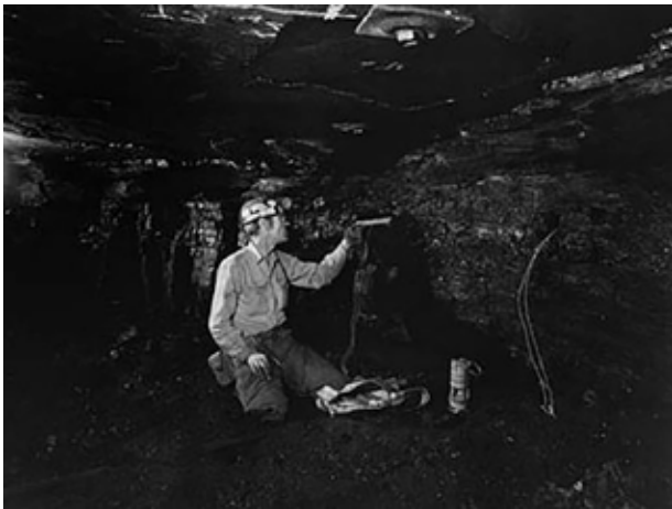
Loading a drill hole underground
