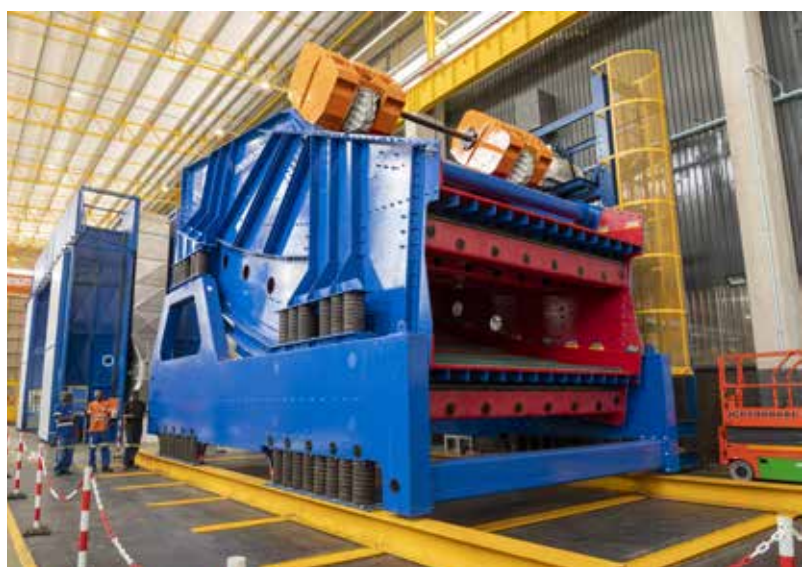
ENDURON Elite screen during assembly, engineered for durability, precision and long service life in demanding mining applications.
