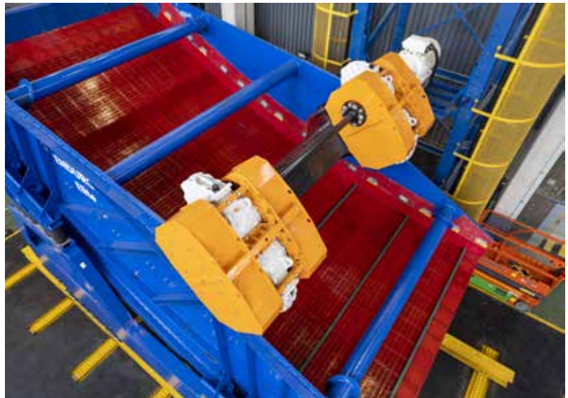
The ENDURON Elite's two-exciter drive design reduces mechanical complexity, maintenance demands and operating costs.
